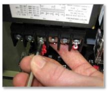
7. Install the extra screw back onto the old PT location and tighten.
