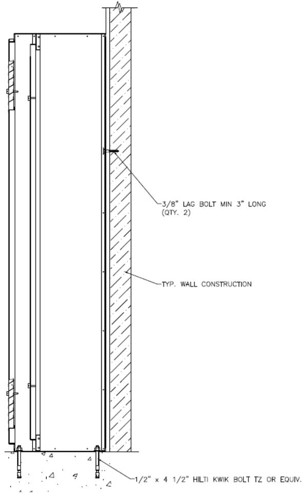
TYP. FLOOR/WALL ANCHORING
