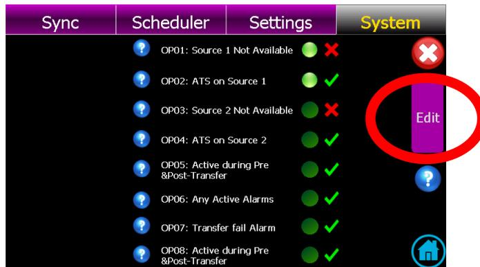
c) With the Output Mapping page displayed, select the desired programmable output # (row) to be edited, then select the desired function for mapping (scroll up or down to navigate to desired function):
