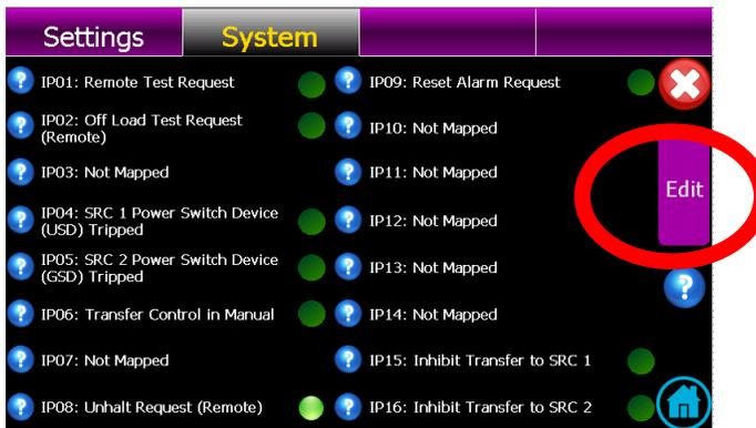
c) With the Input Mapping page displayed, select the desired programmable input # (row) to be edited, then select one of the available USER DEFINED 1-16 functions listed on the right-hand side of the screen. Once selected, use the “Edit” button as shown below.
