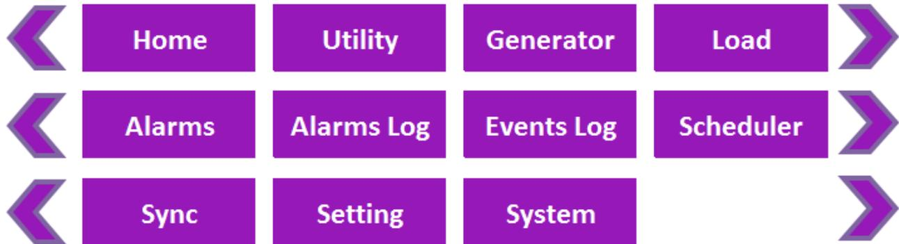
**Note:** the “Sync” page will only be visible for ATS applications that are capable of fast in-sync transfer
